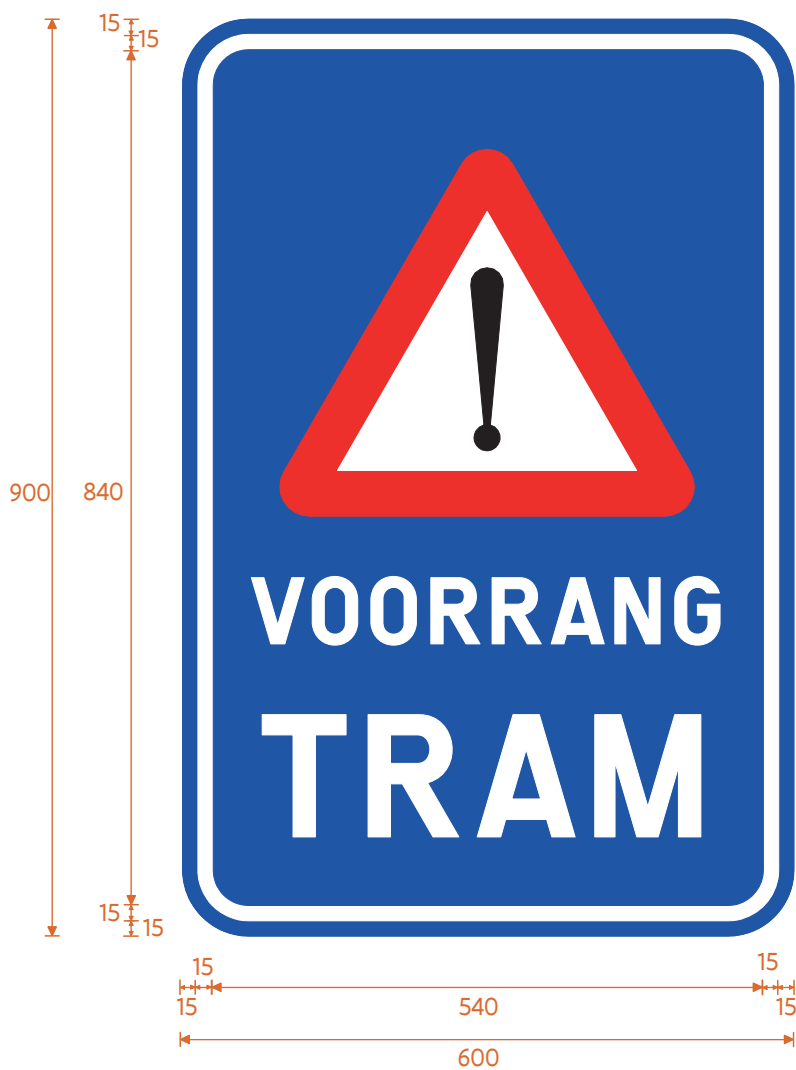
Details bord "voorrang tram" (in mm)
